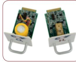
Access through the rear panel allows easy and quick sensor swap for recalibration or replacement in the anaerobic chamber without down time. Sensor calibration data is kept on the sensors so a fast down load of new sensor data to the CAM-12 is all it takes to get accurate measurements.
